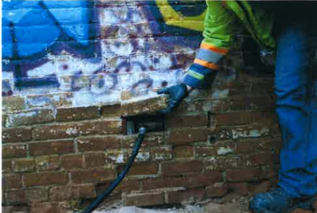
Figure 13 – Detail of testing equipment and brick #1 (Corner building)
