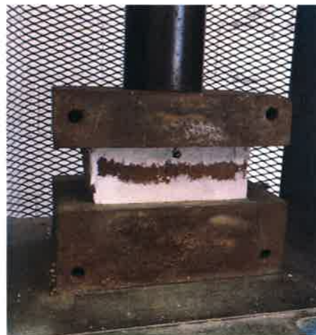
Figure 19 – Specimen #6 (Chimney) before test.
