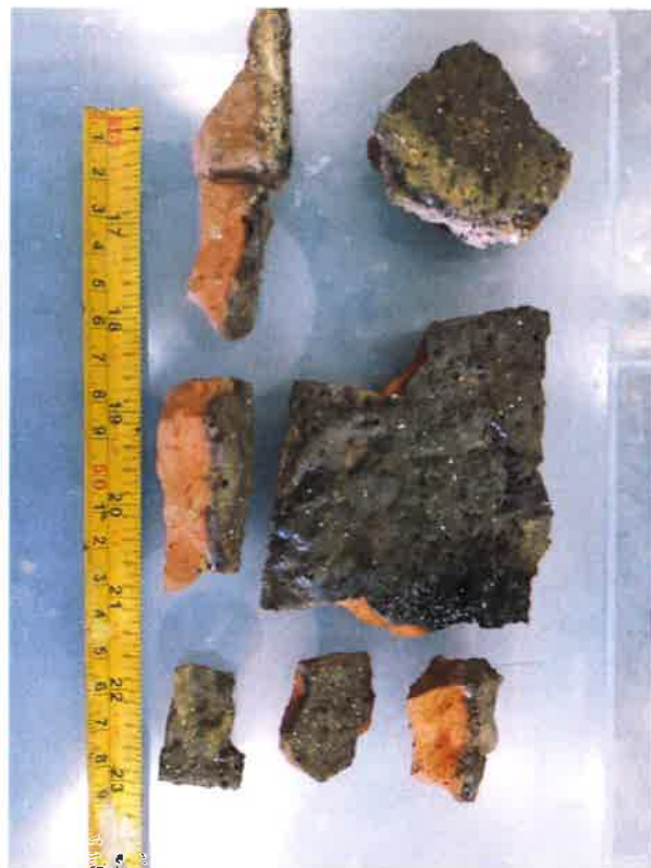
Figure 4 (right) – Detail of delaminated slag and bricks.
