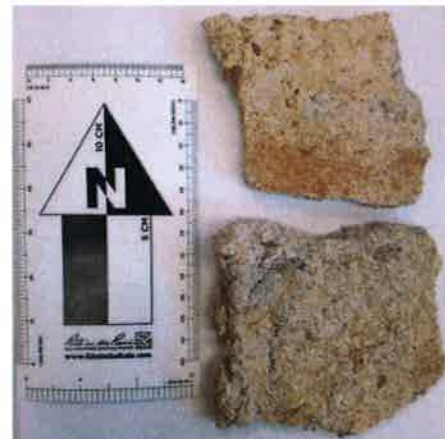
Figure 12 – Lime mortar from Corner Building.
